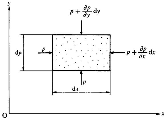
Fig. 12.1 Balance of pressures on fluid element
