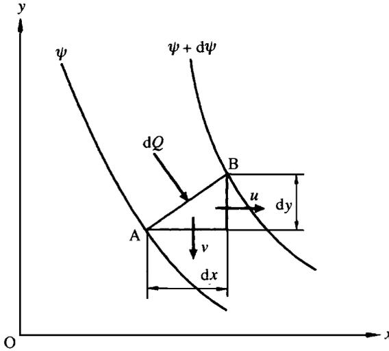
Fig. 12.2 Relationship between flow rate and stream function
