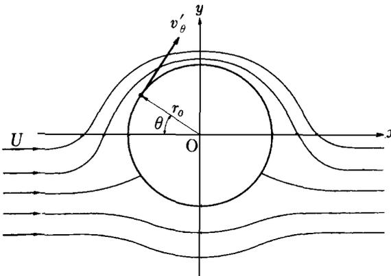
**Fig. 12.12** Flow around a cylinder with circulation
