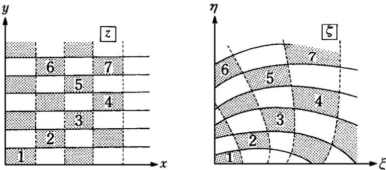
Fig. 12.13 Corresponding mesh on  $\zeta$  and  $z$  planes
